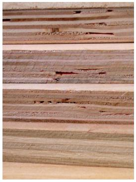
cores are riddled with voids and overlapping layers. The wood is not properly dried; the plywood warps and bows within hours after it is removed from its stack. In the plywood parts used to make the Clamp Caddy, we saw bows of an inch or more over a 24-inch length – and this is typical!
