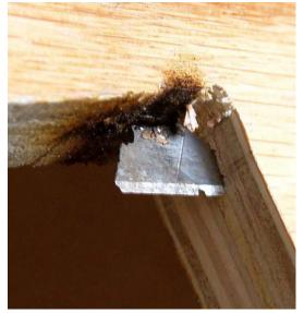
**Above:** A little surprise hidden between the plies of a piece of Chinese plywood. **Below:** Uneven plies, overlapping layers, and collapsed voids in the single sheet of plywood we used to make the Clamp Caddy. And this is the norm! At the very bottom is plywood sold by the same retailer for the same price just two years ago.
