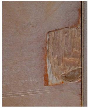
**Above:** This piece of veneer peeled away when we removed a bit of tape. The plies beneath were not properly laminated.
