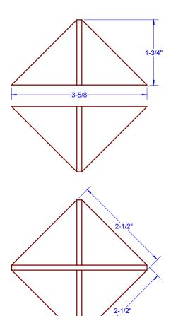
2. Sandwich each narrow rectangular strips between two triangular strips to make two halves.
