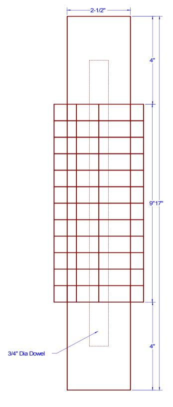
5. Stack the slices on a 3/4"-diameter dowel. Drill 3/4"-diameter holes in the ends of two rectangular blocks. Glue all the parts together with the slices sandwiched between the blocks.
