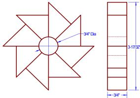
4. Band saw the assembly into 3/4"-thick slices and drill a 3/4"-diameter hole in the center of each slice.
